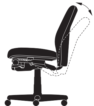
Flexible Back (Free-Floating Synchrotilt) 20° Range (90° - 110°)
