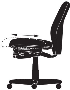
Seat Depth Adjustment (Sliding Seat Pan) 3" Range (16" - 19")
